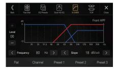
The channel being adjusted is displayed in red.
