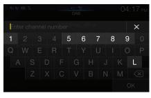
You can enter channel numbers of up to three digits. Each time you enter a number, receivable channels will be narrowed down.
