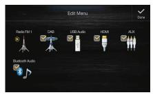
The source icon displayed in the Edit Menu screen is displayed only when usable setup and conditions of each Audio source are fulfilled. For details on setup and conditions of each audio source, see "Switching Sources" (page 15).
