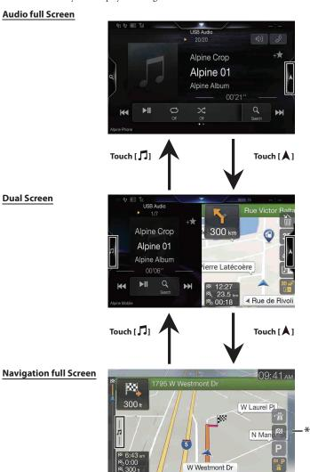
\* Touch [🔍] to switch to the Navigation menu screen. For details of navigation operations, refer to "Navigation System OM" in the CD-ROM.
